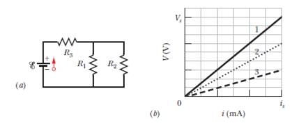
56. Line 1 has slope  $R_1 = 6.0 \text{ k}\Omega$ . Line 2 has slope  $R_2 = 4.0 \text{ k}\Omega$ . Line 3 has slope  $R_3 = 2.0 \text{ k}\Omega$ . The parallel pair equivalence is  $R_{12} = R_1 R_2 / (R_1 + R_2) = 2.4 \text{ k}\Omega$ . That in series with  $R_3$  gives an equivalence of
